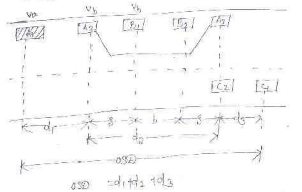
d, -> distance travelled by overtaking vehicle in reaction time. (In this . time the vehicle 4) is force to move with slower speed he vy. d, + VB x tr (Asper Irc tr = 2 sec) do -> distance travelled by over taking vehicle while accolerating do = Vb · T + f at2 - 490 do = bt 28 b -> dispunce Aravelled by overtaken vehicle. da - VIT + 18 --- (1) cq" Equating egn () and egn () NA + + + + = = NA + = 8 7 - 143 S : min space interval both two. vehicles
