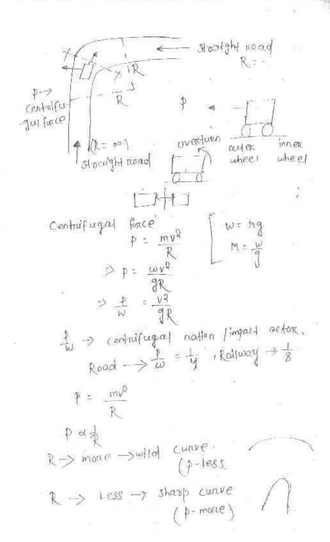
TOKING moment of force with respect to outer wheel when vehicle is just about to overturn,
