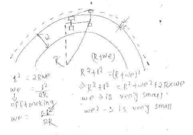
on a no of between lones A : = Length of arts of the vehicle - om! R = Radious of curve wm = mechanical windening: psychological widening :-- 000 -- S WPS = 1 V → speed in kmlh R > Radious inmi We - n12 + v 2R + 9.5rR
